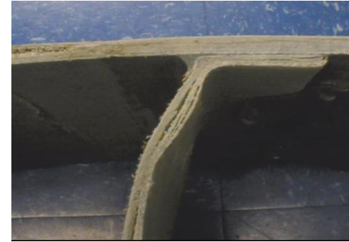
Type 6: Buckling of main spar and disbond as result
