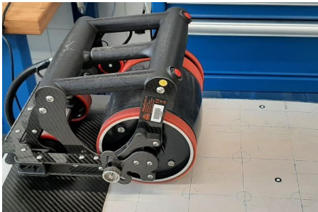
0.5 MHz Roller probe
