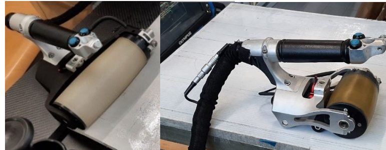
1 MHz Roller probe
