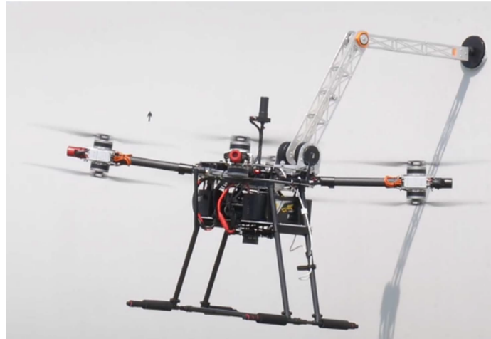
Fig. 1: Snapshot of Sarax, the proposed Aerial Manipulator platform, during a physical interaction task.
